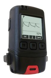
The GFX-T standalone USB data logger measures and stores up to 252,928 temperature readings over a -30 to +80°C (-22 to +176°F) range and at a resolution of 0.1°C.
