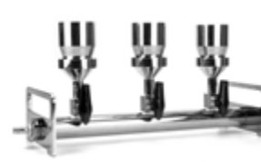
3-branch Stainless Steel Manifold set ( 100ml, 300ml, 500ml ) Order No.: 167103-24, 167101-23, 167101-24
