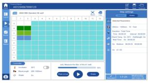
The built-in software of FlexA-200 which has 10 inch high resolution touch screen and adopts the graphic interface, it makes the operations easy. In addition, you can use USB to export data
