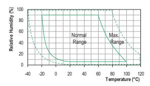
Long term exposure to humidity levels outside of the 'normal' range may temporarily offset RH measurements ( $\pm 3\%$ RH after 60 hours). Once returned to less extreme conditions the device will slowly return towards calibration state.
