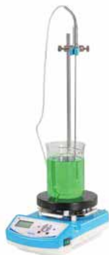
Magnetic stirrer to measure liquid temp.
