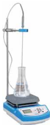
Magnetic stirrer to measure liquid temp.
