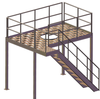
Operating platform 100L to 200L
